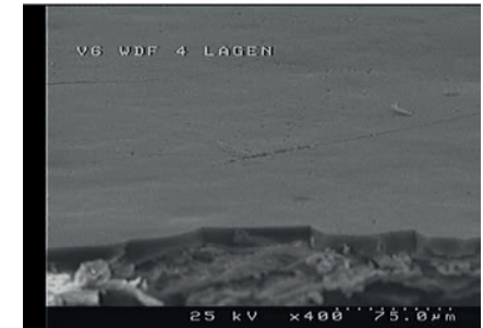
Dry toner layer of 4 colours melted onto a paper label substrate showing the particle behaviour has completely disappeared.
